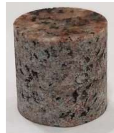
1 cm diameter core sample
