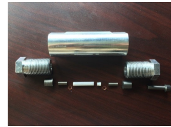
Clamp cells for up to 2 GPa at ultra-low temperature and high field
