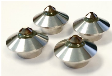
6 mm conical CVD anvils inside steel seats.
