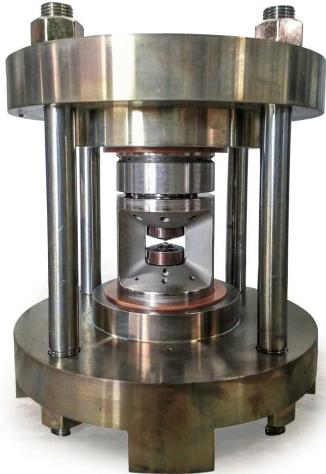
Panoramic diamond cell inside a membrane press. The sample volume was \sim 0.05 \text{ mm}^3 [1].
