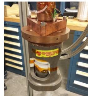
Uwatoko palm-cubic cell for up to 7 GPa
