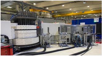
A **dedicated** diffractometer optimized for extreme conditions (**high P, high H, low and high T**) but with **flexibility** to accommodate a broad range of studies
