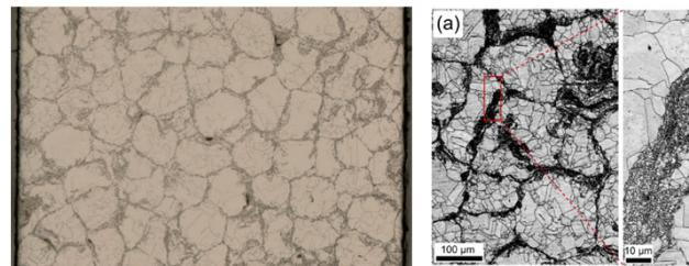
Coarse grains embedded in skeleton of ultrafine grains
